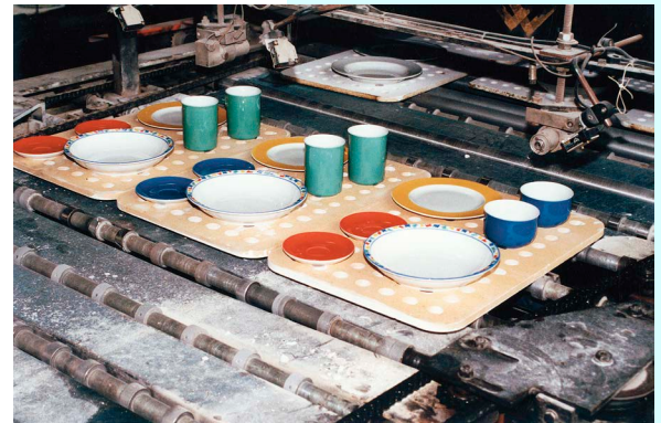
Plate for firing tableware in roller kiln
